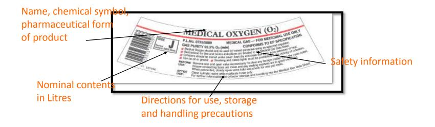
The contents stated on the cylinder collar should correspond with the colour of the cylinder.
