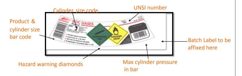
Cylinder collar labels give important safety and usage information, as well as confirming the identity of the cylinder contents. They should ALWAYS be checked before a cylinder is used and should NEVER be removed.
